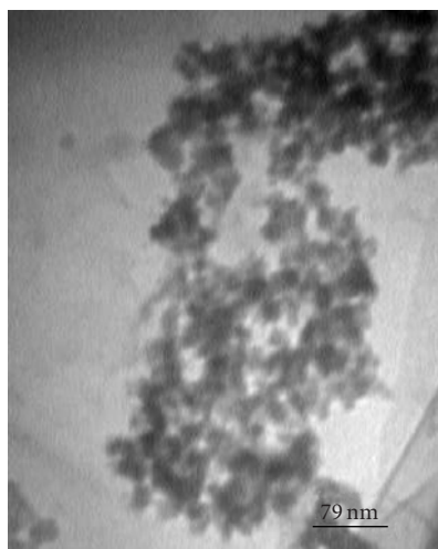
FIGURE 6: TEM image of the NiO nanoparticles (PEG 1 g).
