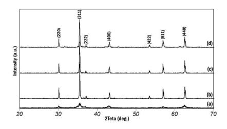
Fig. 1. X-ray diffraction pattern of the samples: (a) milled for 20 h, (b) milled for 20 h then annealed at 750°C for 2 h, (c) milled for 20 h then annealed at 750°C for 2 h with NaCl:CoFe<sub>2</sub>O<sub>4</sub> ratio of 4:1 and (d) milled for 20 h then annealed at 750°C for 2 h with NaCl:CoFe<sub>2</sub>O<sub>4</sub> ratio of 10:1.
