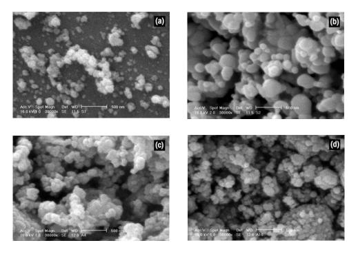
Fig. 2. SEM images of the samples: (a) milled for 20 h, (b) milled for 20 h then annealed at 750°C for 2 h, (c) milled for 20 h then annealed at 750°C for 2 h with NaCl:CoFe2O4 ratio of 4:1 and (d) milled for 20 h then annealed at 750°C for 2 h with NaCl:CoFe2O4 ratio of 10:1.
