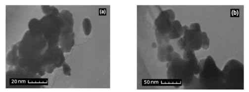
Fig. 3. TEM images of the samples: (a) milled for 20 h, (b) milled for 20 h then annealed at 750°C for 2 h with NaCl: CoFe2O4 ratio of 10:1.
