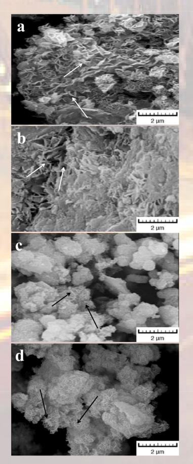
Fig 2. SEM micrograph of the NiO powder synthesized by the TSSC at: (a) 22, (b) 32, (c) 55, (d) 75 degrees Celsius. The arrows highlight wall-shaped NiO nanoparticles.
