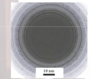
Fig 4. Diffraction pattern image of the produced nanopowder.
