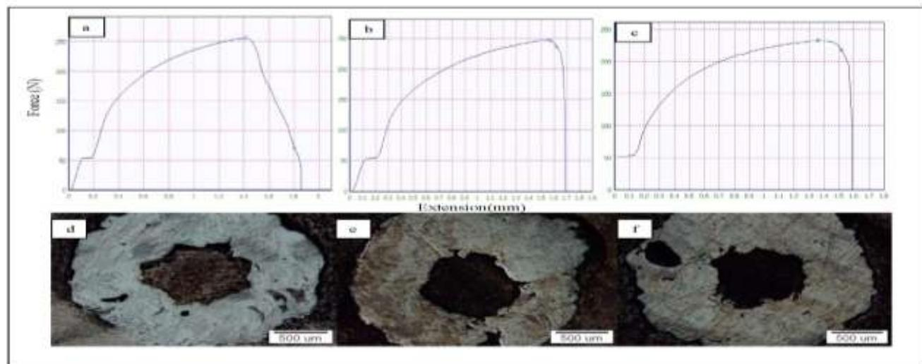
**Figure 7 : Shear force vs. extension in addition to weld seam shape, at bottom interface surface of Ti sheet for samples 4,5, and 6 respectively : a,d. sample 4; b,e. sample 5; and c,f. sample 6**
