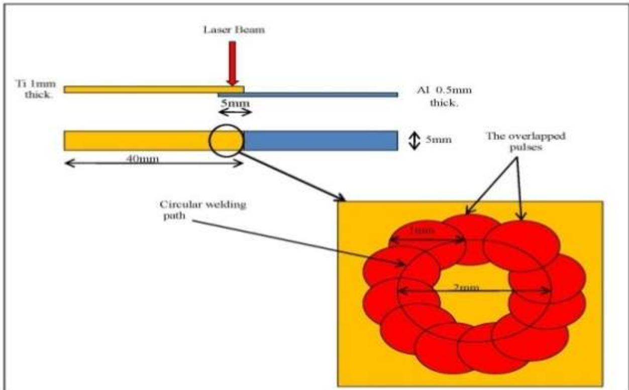
**Figure 1: Joint design and welding Path**
