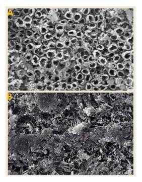
Fig. 3 Scanning electron micrographs of A) TNT B) HATNT
