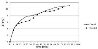
Fig. 5. Temperature increase of pure  $NiFe_2O_4$  nanoparticles after 2 hours of calcination and  $NiFe_2O_4$  - chitosan nanoparticles as a function of time
