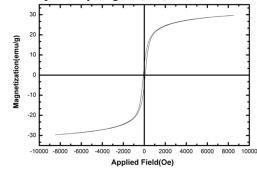
Fig. 3. The magnetic properties of NiFe2O4 - 2h of calcinations
