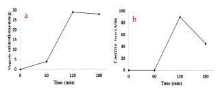
Fig. 4. Changes in specific saturation magnetization with the degree of calcination time (a) and changes in coercivity with the degree of calcination time (b).
