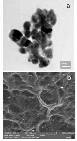
Fig. 1. SEM image of pure NiFe2O4 nanoparticles (a) and FESEM image of NiFe2O4 – chitosan (b)
