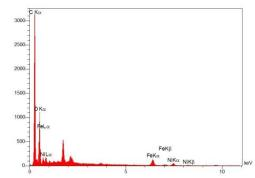
Fig. 2. EDS analysis of NiFe2O4 nanoparticles in figure 1 (b)
